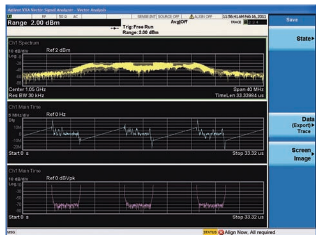
Figure 3. The 89600B VSA software enables analysis of pulsed UWB signals in the time, frequency and modulation domains.
